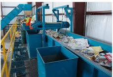
This smaller MRF, located in Bedford County, VA, has a sliderbed sorting line conveyor fed by a combination chainbelt conveyor.
