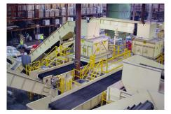
EZ-TRAX Conveyors fit many applications, such as this MRF in Lakeville, MA. It features dozens of sliderbed conveyors, sorting lines, sorting bins, platforms, and baler feed combination steelbelt conveyors.
