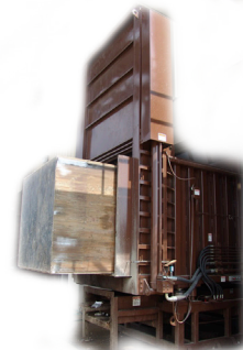
The BlokPak has a 5-foot 1,5- meter ram penetration. This ejects the final log into the trailer with very little spillage.
