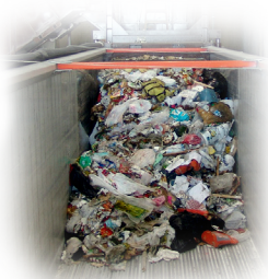
The BlokPak forms 10-foot (3-meter) logs of densely packed waste.
