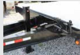
Single Leg Manual Crank, 10,000 lb. Lift Capacity Landing Gear (15,000 lb. static load capacity)
