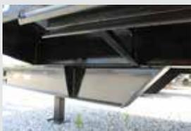
Main Frame is wide flange 10" I-Beam & Outer Frame Constructed of (2) 5" Channels
