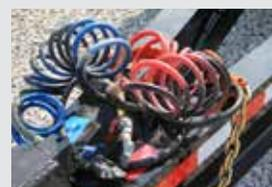
3/8" DOT Service & Emergency Air Lines w/ Glad Hands, (7-round pin "pigtail") Electrical Trailer Plug and Safety Chains
