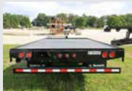
LED lighting: Perimeter/Marker, Running, Stop, Turn and Mid-Body
