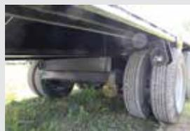
20k lb. Suspension (10 - leaf springs) - 10,000 lbs. Capacity Axles
