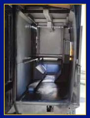
Safe horizontal ram eject unloading eliminates costly multi-stage cylinders. Hardox® wear plates and secondary reinforced welds makes the CS9200SB one of the toughest split bodies on the market.
