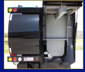
The 40/60 split body features two individual compartments with simultaneous packing and independent compartment horizontal unloading.
