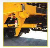
Hydraulic lines are neatly contained and tucked away during arm retraction.
