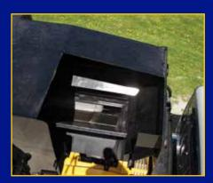
The 50/50 split hopper includes a hydraulic crusher panel that keeps refuse and recyclables or two types of trash separated.
