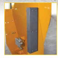
Featuring Nylatron® non-lube wear guides—horizontal slide guides are replaceable without track disassembly.
