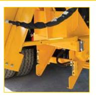
Lift arm service prop allows for safe, convenient and efficient maintenance.
