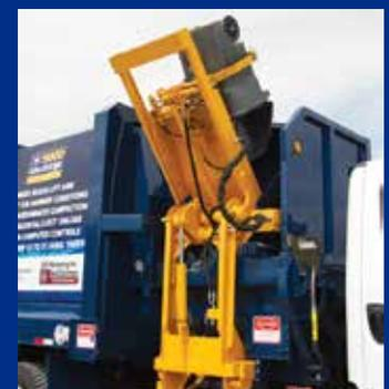
Fast cycle times, continuous packing and a 50 degree minimum dump angle
