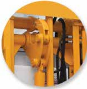
Maximum of only three grease fittings on lift arm and four on the body makes lubricating quick and easy.
