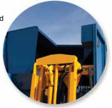
Lift arm service prop allows for safe and convenient maintenance.
