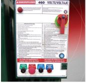
Standard controls: key lock On/ Off Auto Cycle, Emergency Stop, and Platen Raise/Lower. A Baler Ready light indicates the baler is operational. Also available with "Bale Made" light and electrical disconnect (shown).
