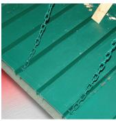
The standard chain bale ejector is manually set after the bale door is opened.
