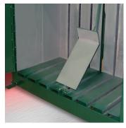
An optional automatic bale ejector is also available. It is actuated when the bale door is opened.
