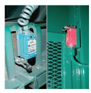
A redundant interlock system is incorporated into the feed gate switch.
