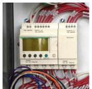
If there is an attempt to override the interlocks; the panel box features a programmable "smart" relay control system that disables the baler. The relay add diagnostic and trouble-shooting capabilities.
