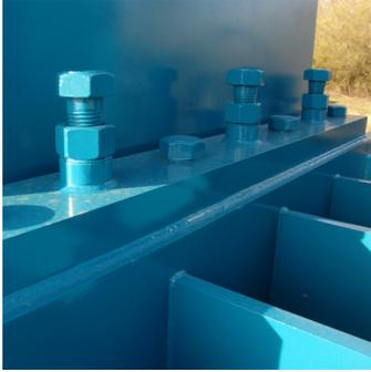
The Galaxy2R® narrow model features an adjustable shear beam that enables you to adjust the shear blades from the exterior of the machine.
