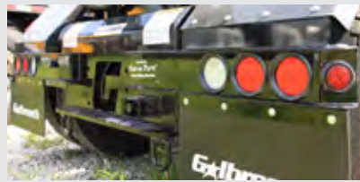
HD rear apron that is pintle adaptable with back up alarm and split bumpers with LED lighting and mud flaps
