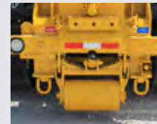
Rear hydraulic stabilizer with 10" ground roller
