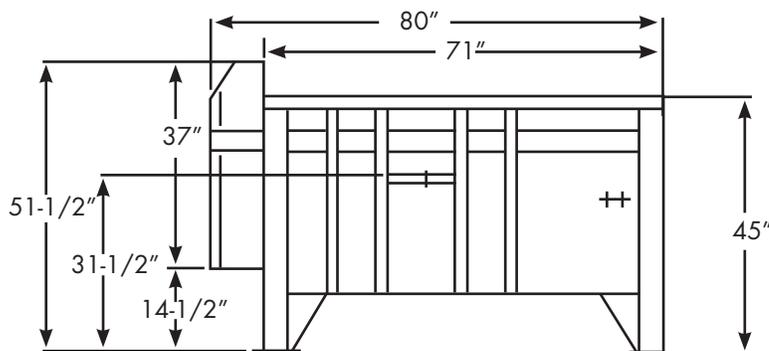
K-PAC “Stubby” compactors are manufactured in fixtures to ensure concentric and consistent equipment every time. A superior paint finish is applied using a modified acrylic enamel with high UV protection. After application the paint is baked on to ensure proper cure for exceptional durability. A clear chamber opening of 41” x 57” will handle most industrial needs. A full 13” of ram penetration with built in breaker bar teeth provide compaction exceeding competitive models.
