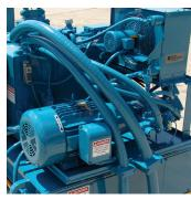
TEFC motor with quiet running pump system.
