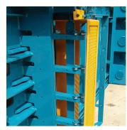
Wire postioners are on the twister cabinet side for precise twister alignment and wire pick-ups.
