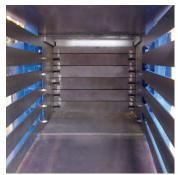
Wear resistant, replaceable Nylatron liners on the ram slides. 500 Brinell steel liners on the floor and ram bottom. Oversized ram hold-down bars are adjustable from the exterior of the machine.
