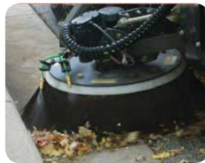
"open throat" suction nozzle design reduces clogging and plugging associated with leaves, twigs, mud, bricks and broken pavement.
