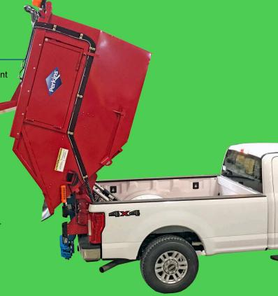
This 6 yard SAT is equipped with a sweep lid and grabber lifter.
