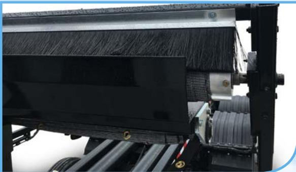
Optional trash brush closes the gap between stabilizer bar and tarp roller.
