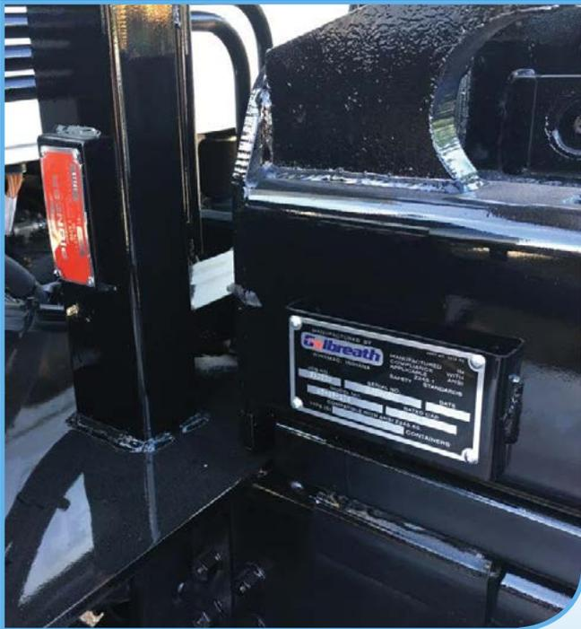
Riveted-style serial number plate allows for permanent identification of a unit
