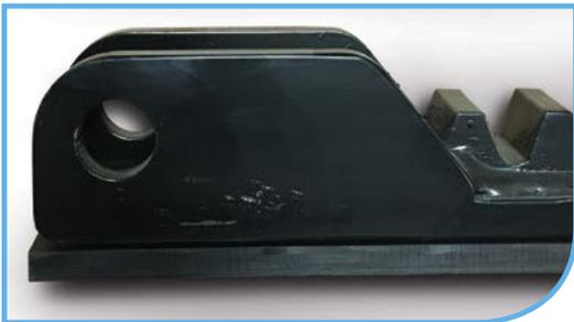
Rack gear weldment eliminates the need for a rack gear cylinder strap and reduces maintenance. A 3/8" self-lubricating polymer bearing is designed to last the life of the arm, but can be easily replaced if needed.
