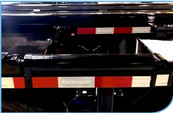
Cylinders mounted externally for maximum accessibility and maintenance
