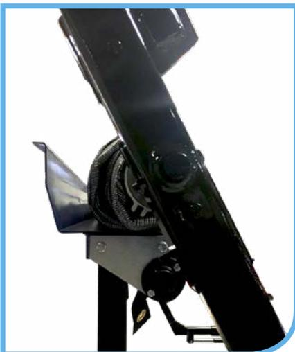
Upper extension arm makes it easier to preload the spring roller and minimize the potential for the tarp roller shaft to seize in the arm bushing
