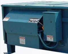
The RJ-275XHD uses a remote power unit with controls that are key-operated and fully automatic. The heavy-duty pushbutton controls are contained in a weatherproof NEMA 13 enclosure.
