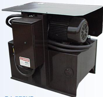
The RJ-575HD features a high-performance remote power unit with a UL and CUL Listed panel box, 30 HP motor, and an external motore starter reset button.
