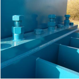
The Galaxy2R® wide model features an adjustable shear beam that enables you to adjust the shear blades from the exterior of the machine.
