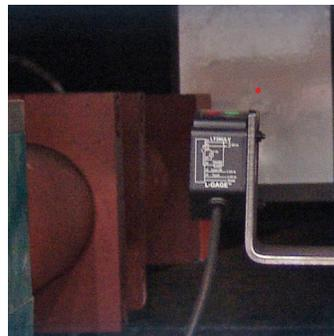
The main ram, ejector ram, and multi-purpose door are controlled by a long range laser sensor. The positioning is determined by the laser and eliminates the need for a counter wheel.
