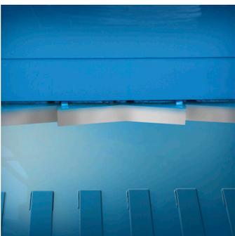
The Galaxy2R wide model ram shear blade is replaceable and reversible. The body shear blade is serrated, adjustable, and replaceable. Replaceable 500 Brinell steel liners on the floor, sides, and platens offer superior wear resistance.
