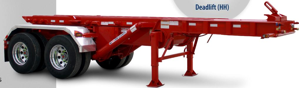
\*EX model shown with following options: aluminum diamond plate fenders, aluminum rims and premium red paint. Standard has black paint, quarter poly rear fenders and steel rims.
