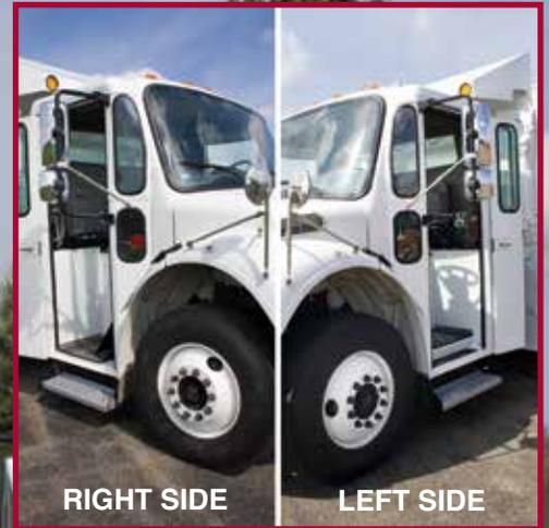
**Independent side loading along with dual stand-up drive cab design allows two operators to work more efficiently.**
